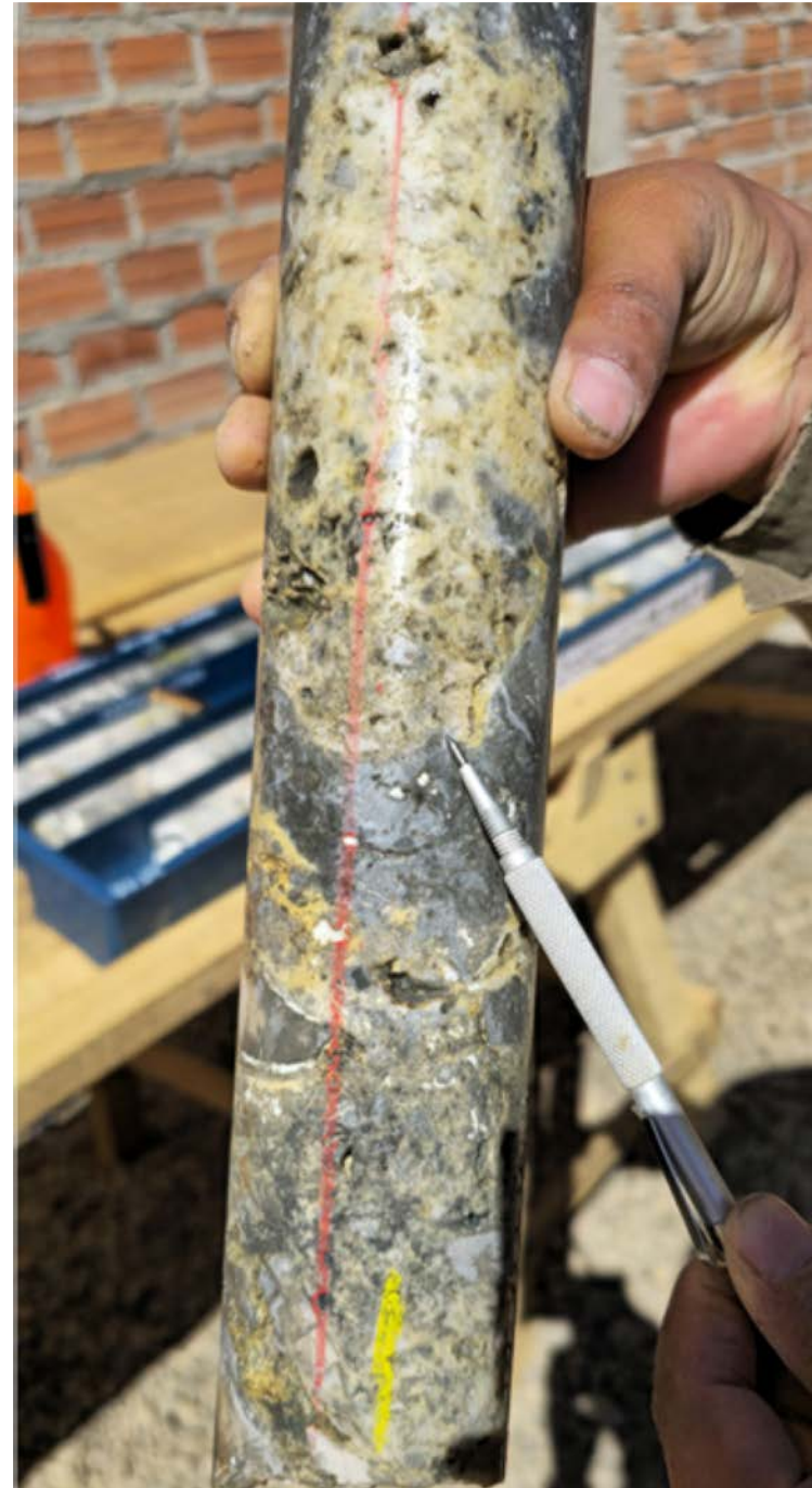
Hole CO-0001: 49.70m, Polymictic breccia matrix supported pervasive silicification with disseminated sulfosalts, local vuggy silica and quartz-alunite-dickite.
